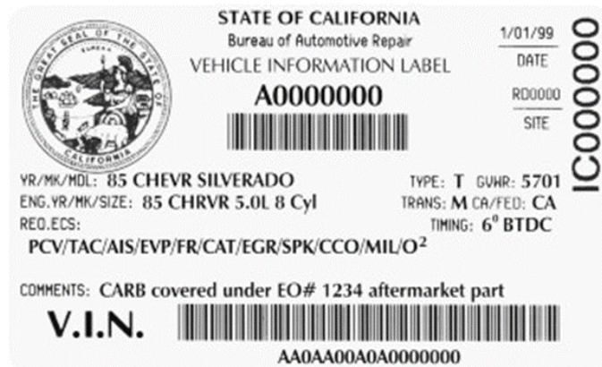
Figure 2: Example of Acceptable BAR Referee Label (all labels must include a serial number)
